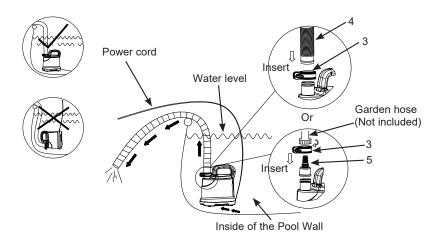
**NOTE:** Maximum pool **water depth** not to exceed 48 in (1.22 m). To protect the pump motor from running dry, disconnect the power cord from the electrical outlet once the water has been drained out or when the remaining water is below the drainage pump base.
