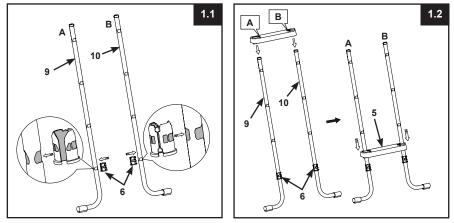
**IMPORTANT:** Ensure the J-shaped legs are pointing outwards before installing the steps.
